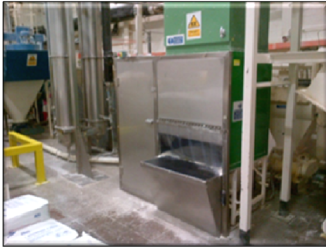
Example 1: Enclosed bag tip with LEV and curtain
