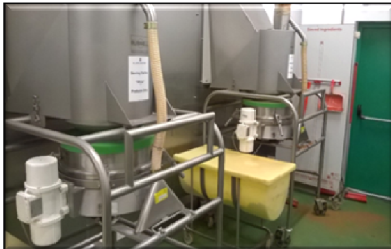
Example 8: Sieving station with LEV at outflow
