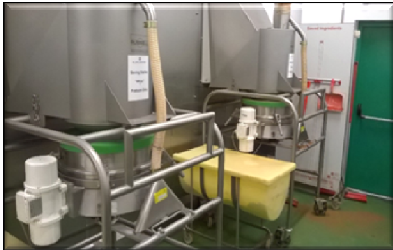
Example 8: Sieving station with LEV at outflow
