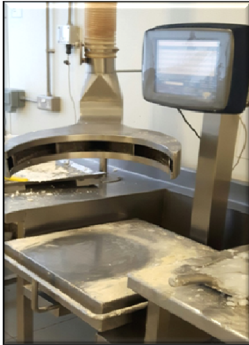
Example 7: Weighing station with lip extraction at tub height
