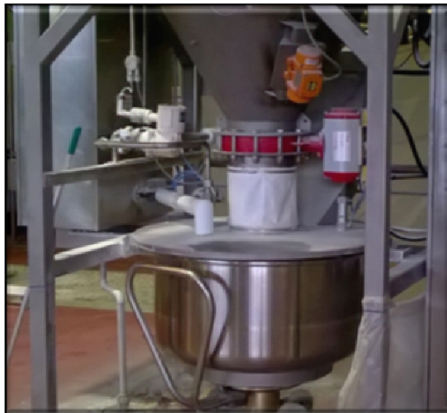
Example 3: Enclosed bulk ingredient dispense
